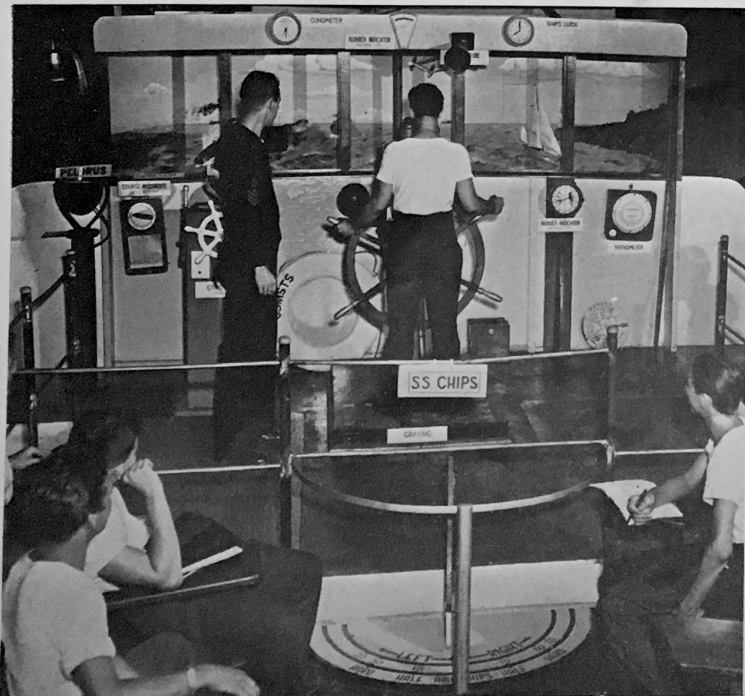
MOCKUP of a complete bridge, the SS Chips provides classroom instruction in the location and use of all equipment and instruments on a ship's bridge.
