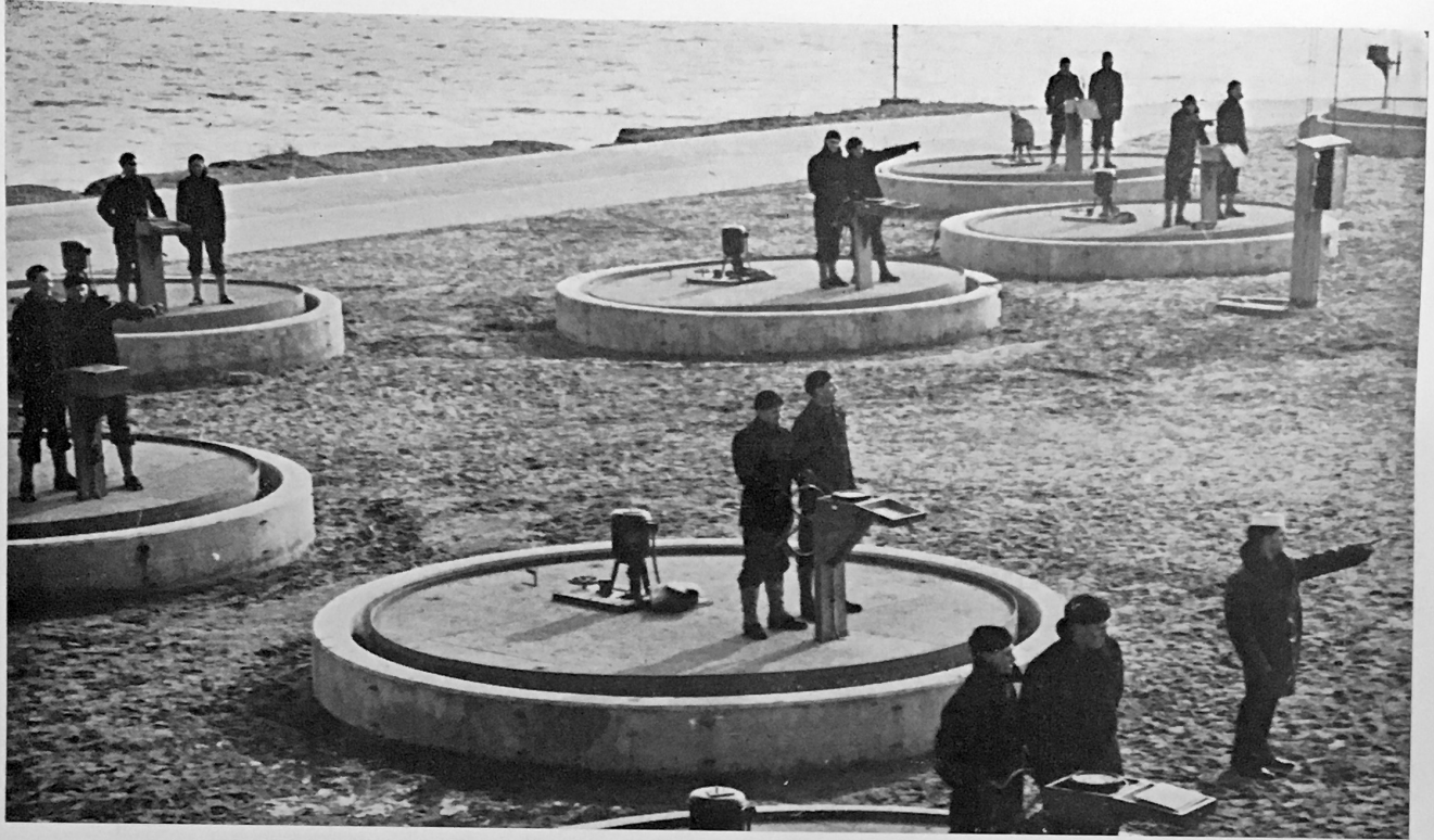
STEERING TRAINERS give trainees the "feel" of steering a compass course. The steel platform, pontoon design, of the trainer pivots in a concrete basin partly filled with water. A small pump drives the water against the platform's keel. As trainee steers a compass course the platform rotates. The device helps overcome the novice's effort to make compass card turn in response to wheel.
