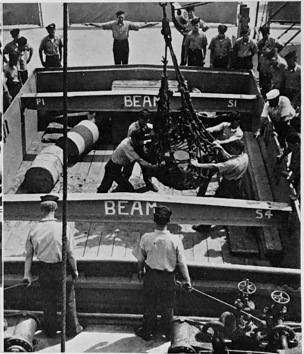
HAND SIGNALS are used to guide winch operators (in foreground) as loaded cargo net is swung by booms from beach into the hold.
