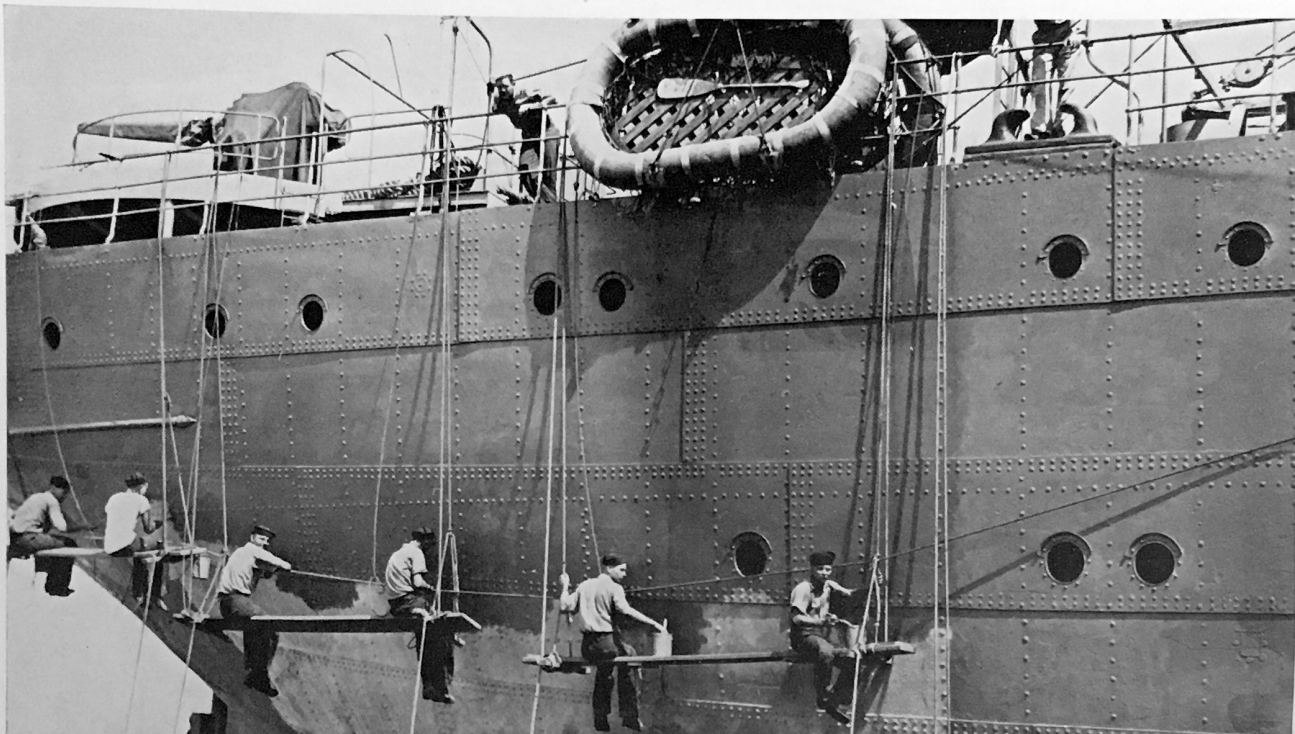
Over the side on stagings to paint the ship gives apprentice seamen practical sample of routine jobs afloat.
