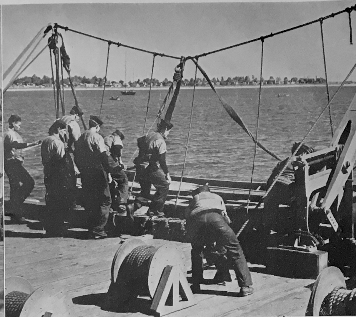
HALF OF CREW springs to lines that lower the boat from davits as rest of crew goes into the boat. As craft is lowered into water this latter group checks all equipment, makes sure everything is set to cast off. Lowering away must be done smoothly and evenly to avoid upsetting boat. When their job on the pier is completed, the men seize the knotted manlines (vertical) and climb down to their boat positions.
